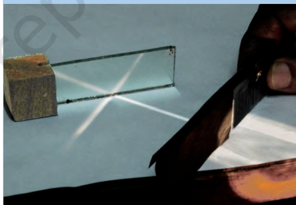
Fig. 16.1 : Arrangement for showing reflection
