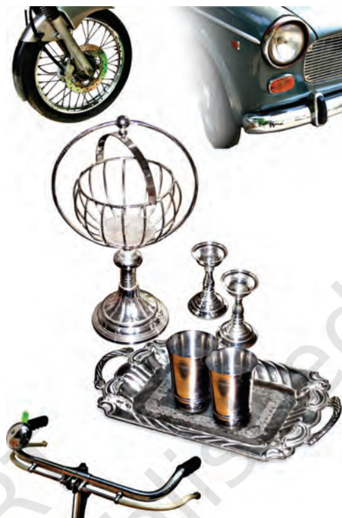
Fig. 14.8 : Some electroplated objects
