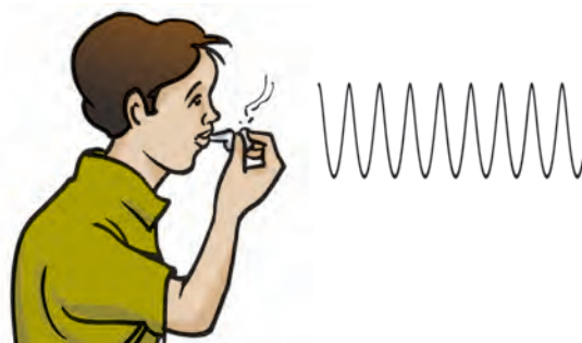
Fig. 13.18 : Frequency determines the pitch of a sound
