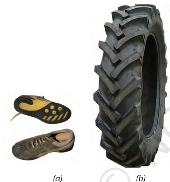
Fig. 12.11 : (a) Soles of shoes and (b) tyres are treaded to increase friction
