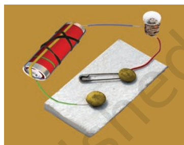
Fig 12.9 An electric circuit with a switch
